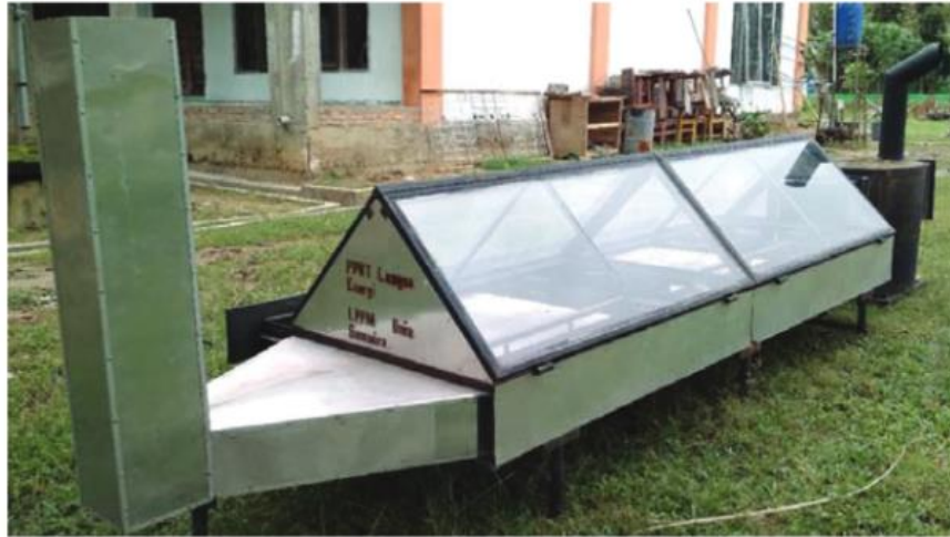
Fig 1.6 Mixed mode type solar drying system [31]
