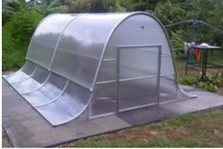
Fig 1.8 PVT integrated drying system[34]
