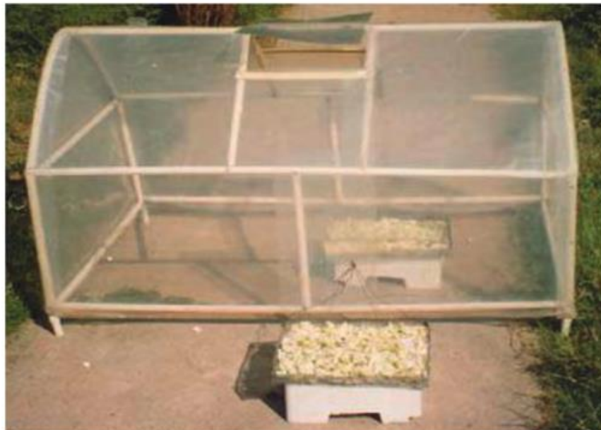
Fig 1.2 Passive greenhouse dryer and the open sun drying [27]
