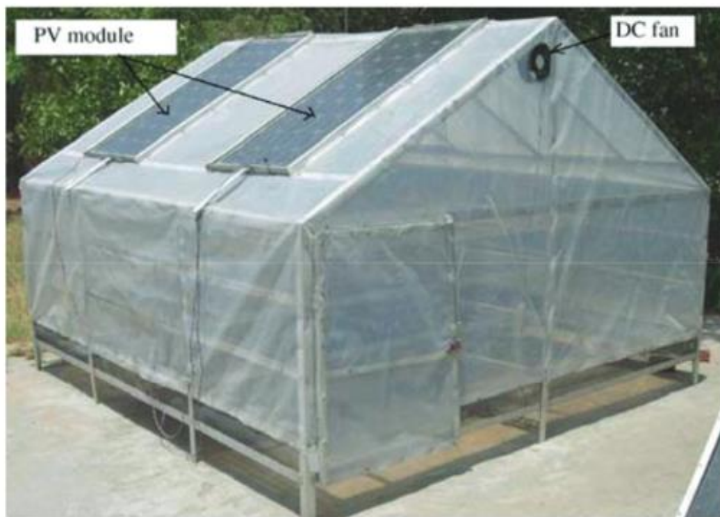
Fig 1.3 Representation of drying sytem operating in active mode [1]
