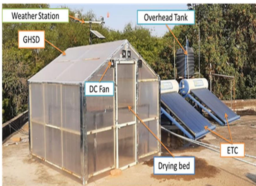
Fig 3.1 Pictorial view of experimental set-up
