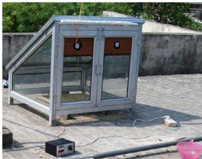
Fig 1.7 PVT integrated drying system [33]
