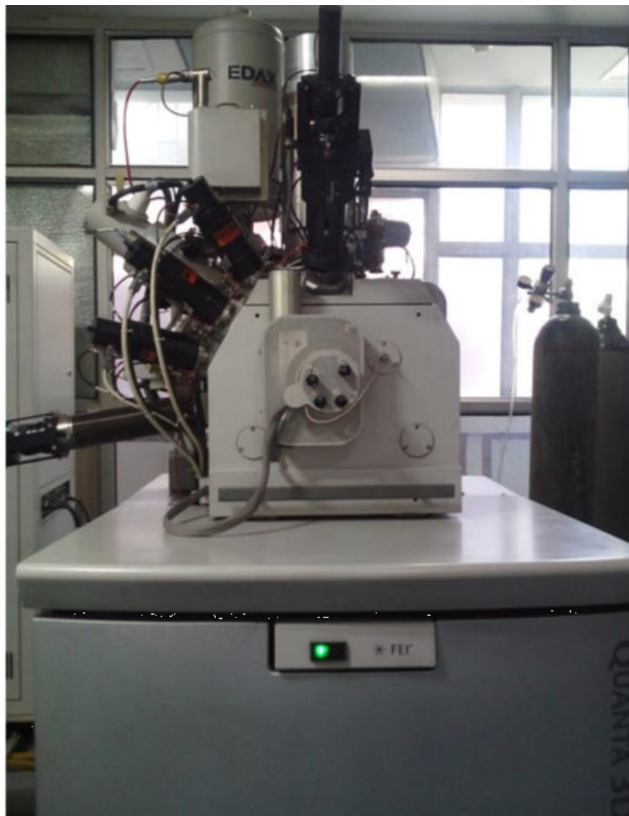
Fig. 3.6 Scanning Electron Microscope with Field Emission Gun (FEG-SEM) (Model: FEI QUANTA 3D FEG)
