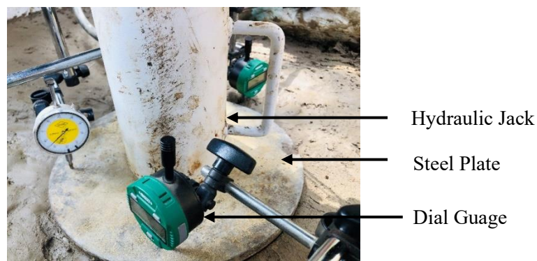
Figure 3.5. Test setup showing various components
