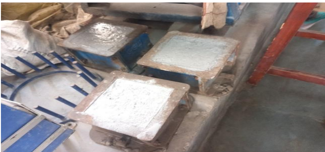
Figure 3.10 Casted Cubes of size 150mm x 150mm x150 mm
