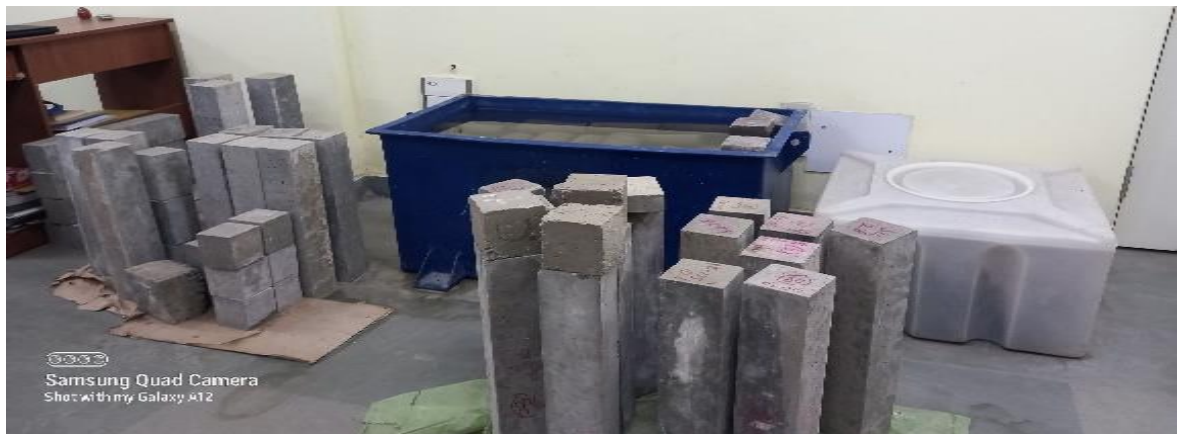
Figure 3.18 Casted beams, cylinders and cubes
