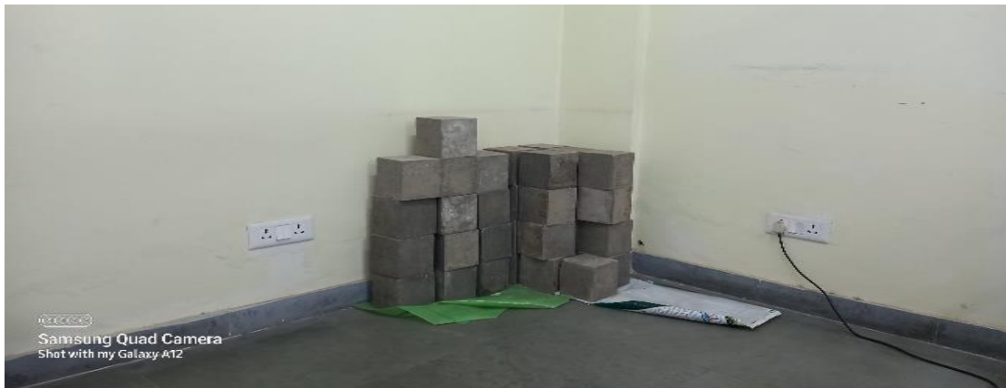
Figure 3.21 Casted cubes of size 150mm x 150 mm x 150mm for water permeability test
