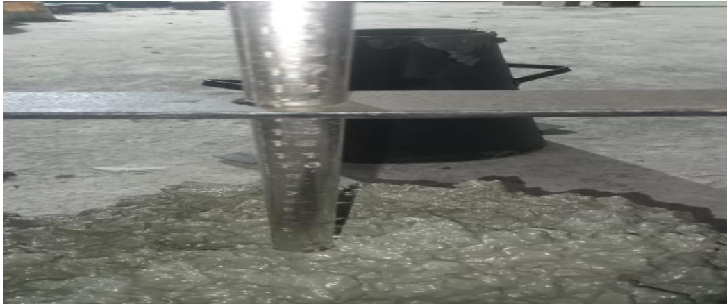
Figure 3.23 Workability Test (Slump Test)
