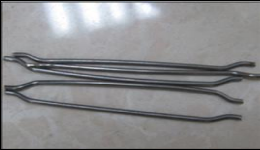
Figure 3.5 Hooked End steel fibres
