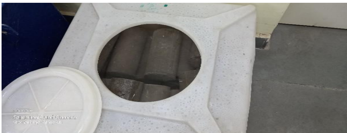
Figure 3.22 Cylinder samples are cured under a water tank.
