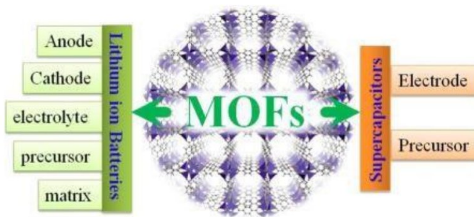
Figure 10: Systematic diagram for MOFs application as Lithium-ion batteries and Supercapacitors.
