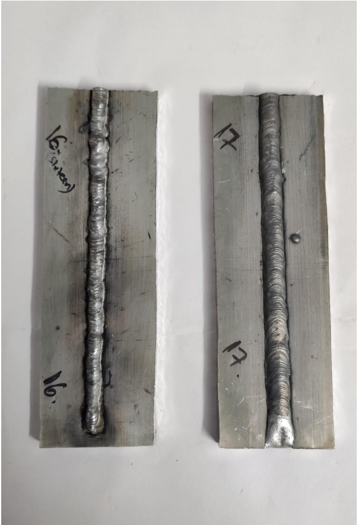
Fig. 5.8: Weld bead obtained by run no. 16 & 17
