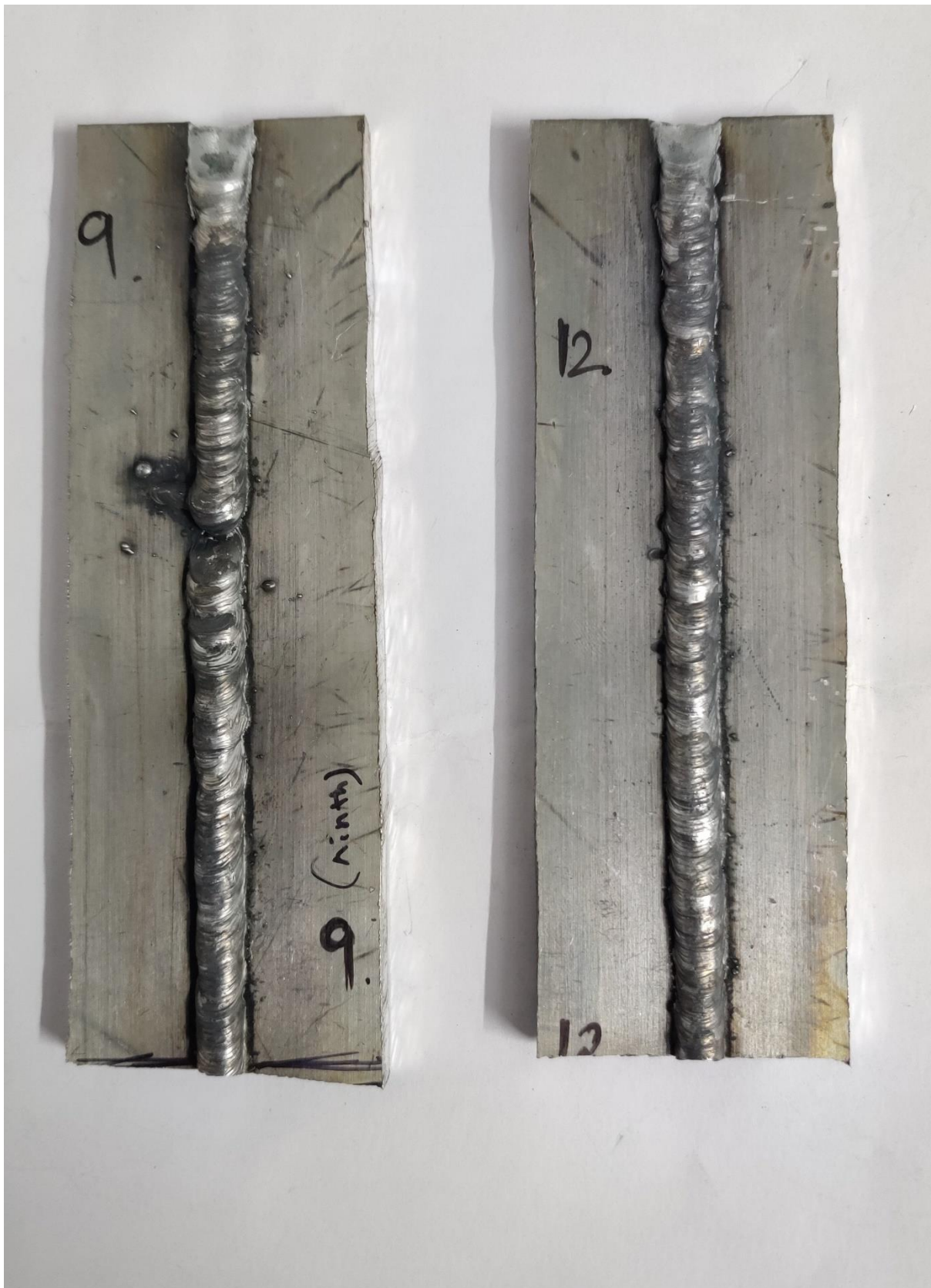
Fig. 5.6: Weld bead obtained by run no. 9 & 12
