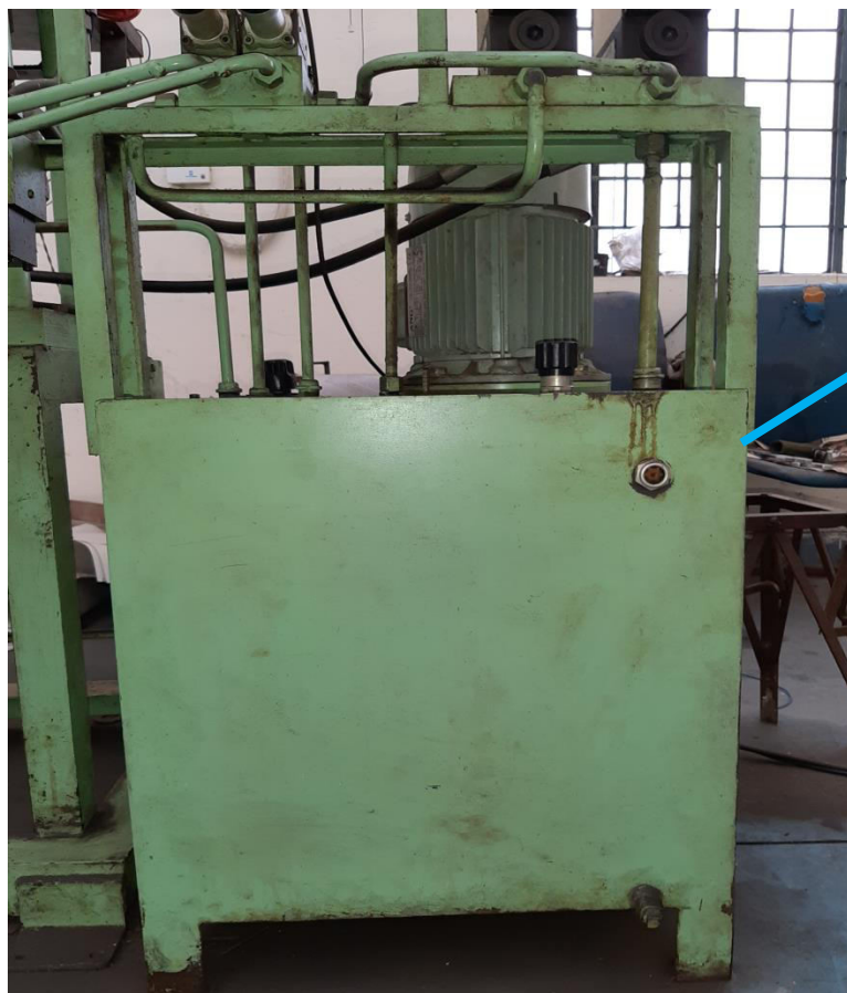
Figure 5.2 Shown Hydraulic Power Pack
