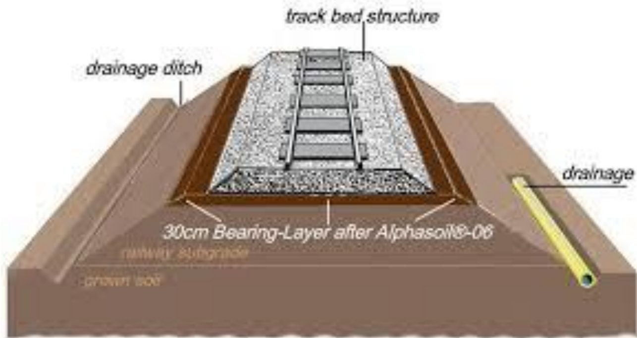
Figure 13: Hydraulically bonded bearing layer
