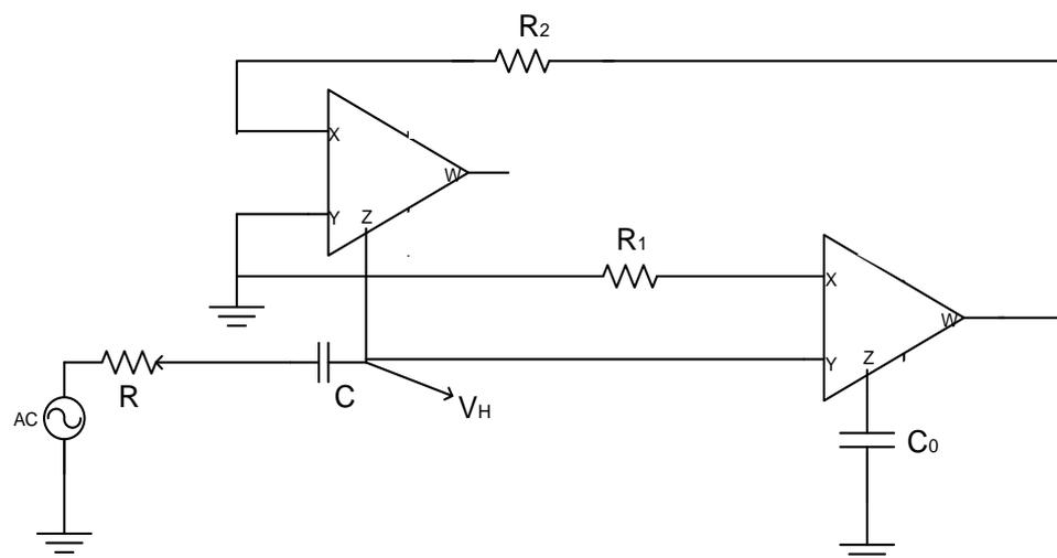
Fig. 4.19 Circuit diagram of high pass filter implemented using GIC.
