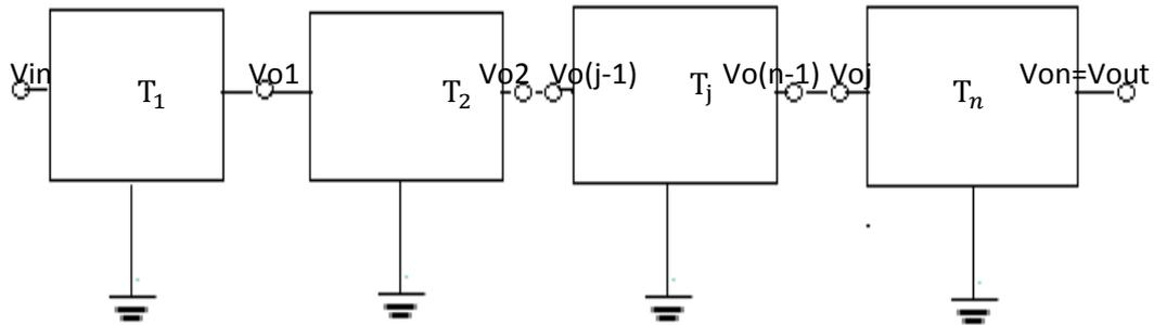
Fig 5.2 Cascade connections of Biquad sections to realize  $n^{th}$  order filter [11]
