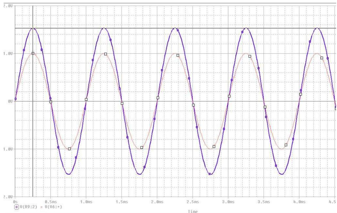
Fig. 4.4 Transient response of SALLEN-KEY low pass filter
