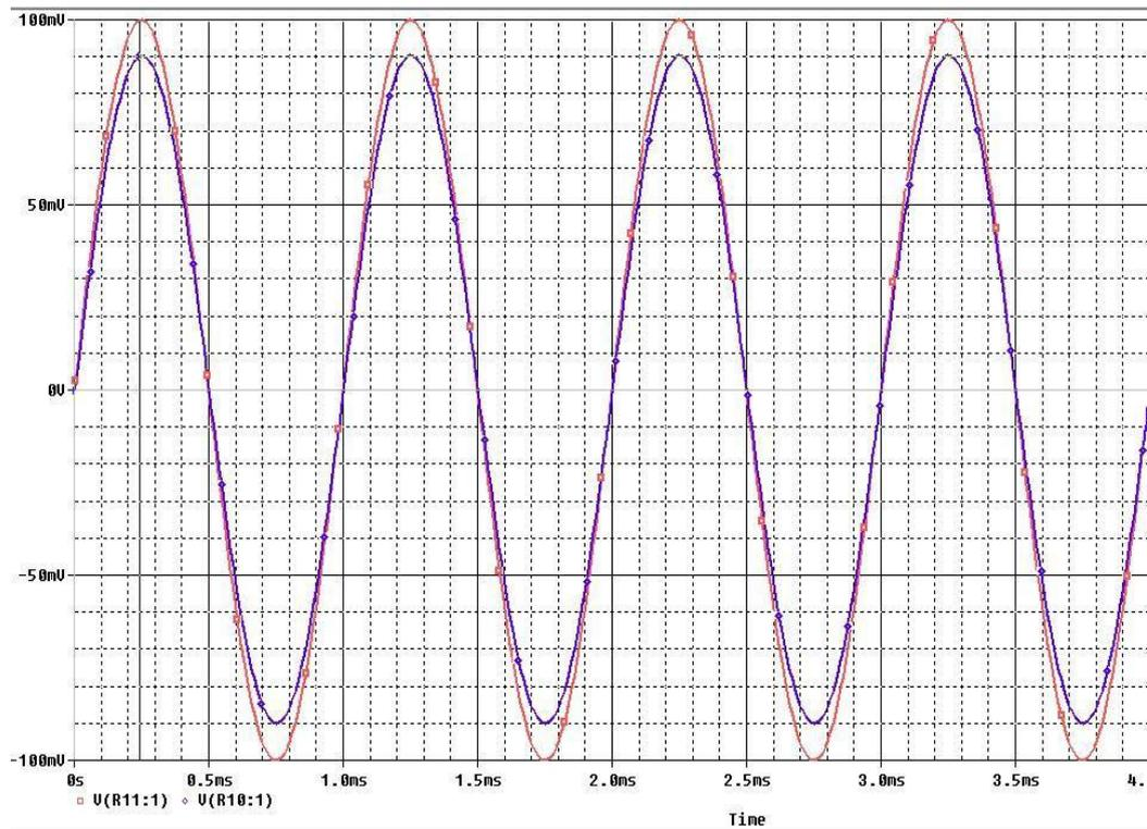
Fig. 3.8 Simulated Transient response of a first order all pass filter
