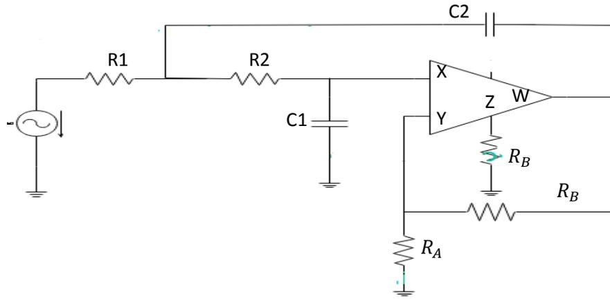
Fig. 4.3 Circuit diagram of SALLEN-KEY low pass filter
