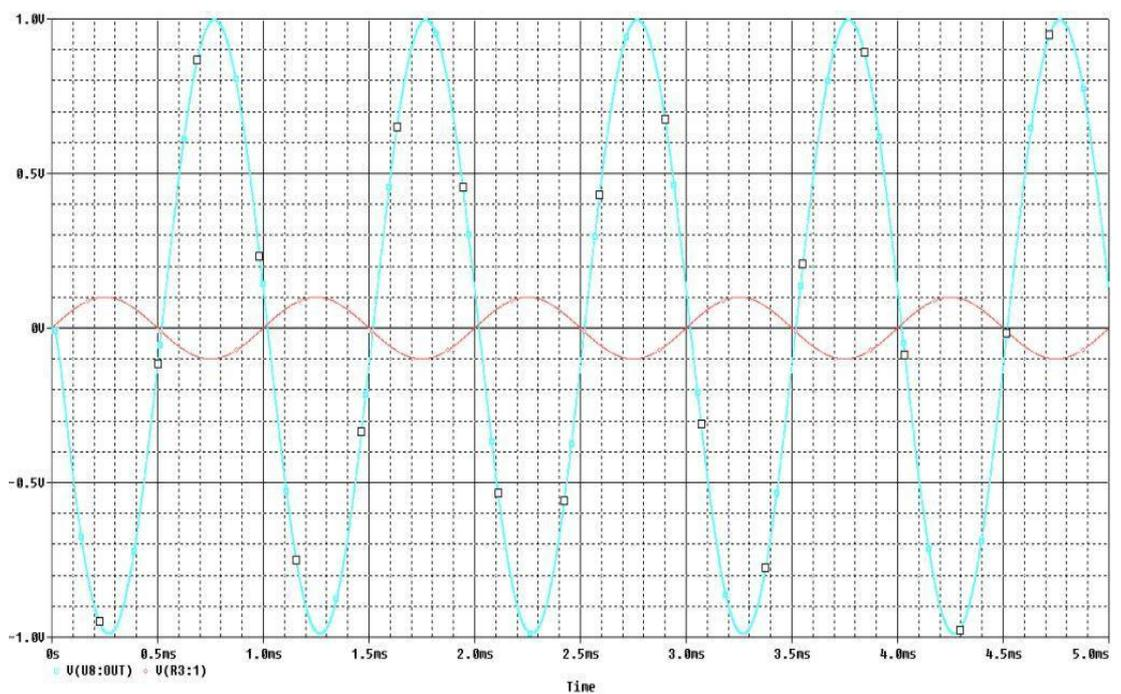
Fig 4.13 Transient response of Tow Thomas Biquad implementing inverting low pass filter.
