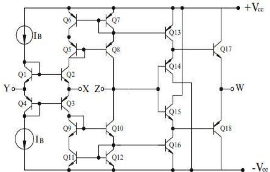
Fig 2.2 Internal Diagram of AD844 (CFOA)
