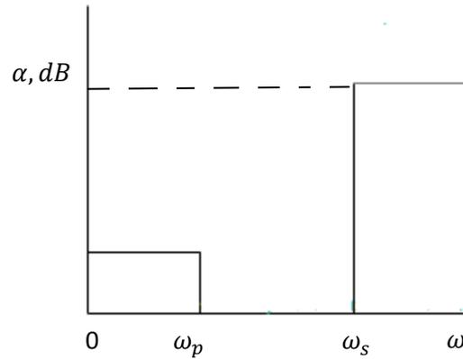
Fig 5.3 Low pass filter specification
