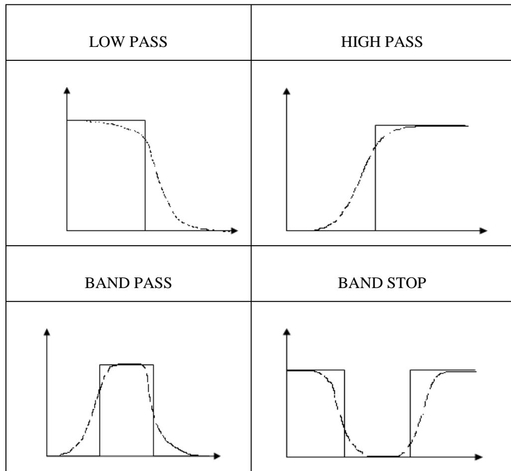
Table 1 Frequency Response of the Four Basic Filter Types. Ideal characteristics;
