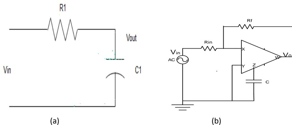
Fig 1.2 (a) Passive Low Pass filter and (b) Active low pass filter.
