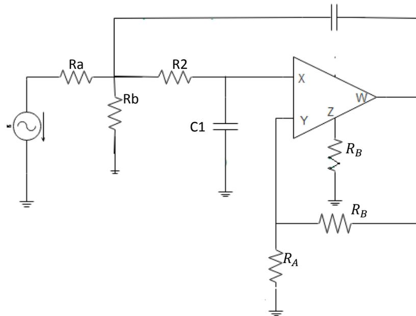
Fig 4.6 Circuit diagram of SALLEN-KEY low pass filter with gain adjustment
