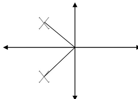
Fig 4.1 Pole locations of second order transfer function.
