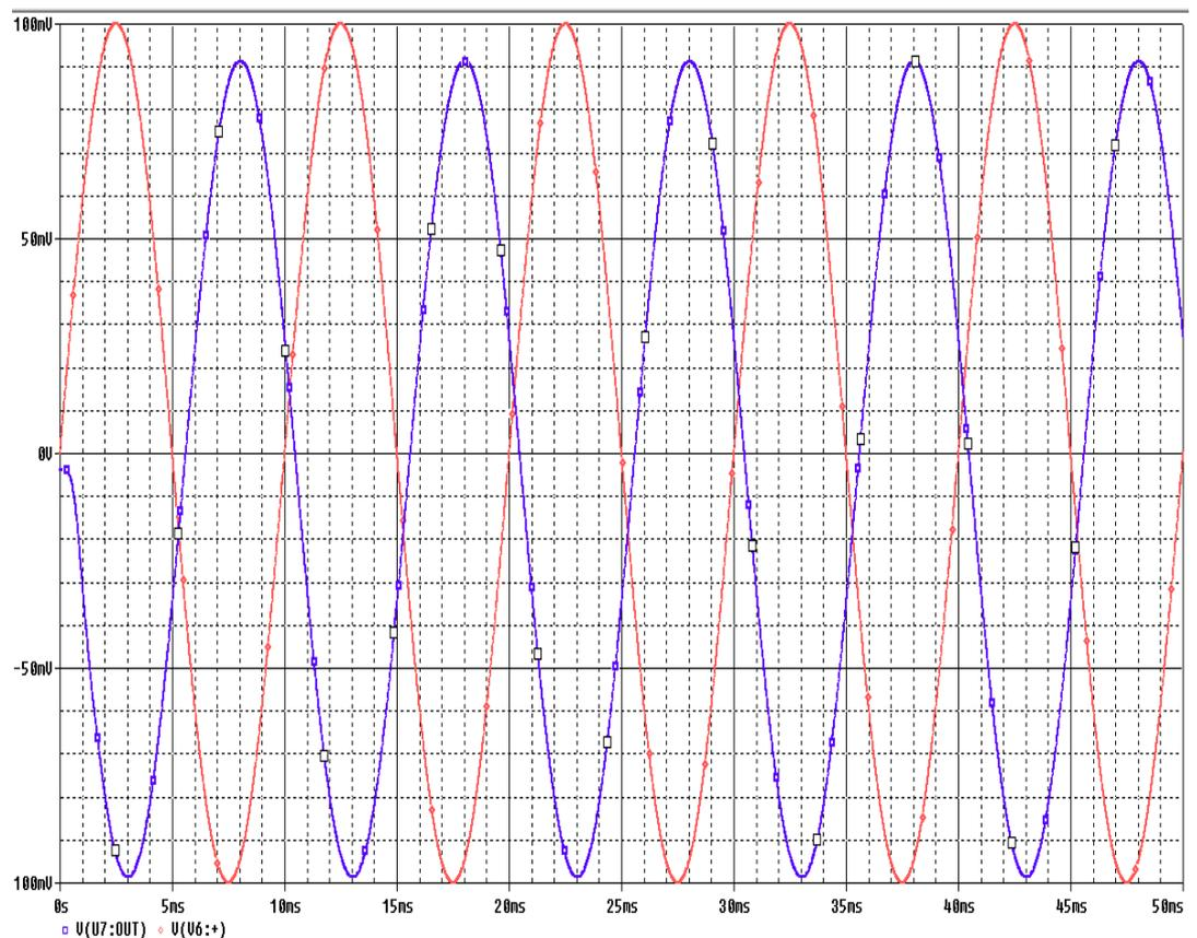
Fig. 5.5 Simulated Transient response of Butterworth fifth order low pass filter
