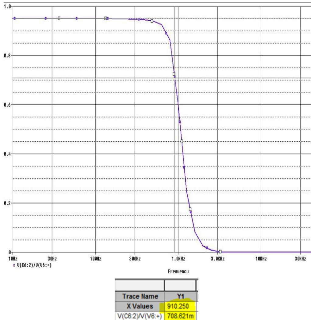
Fig 5.6 Simulated Frequency response of Butterworth fifth order low pass filter
