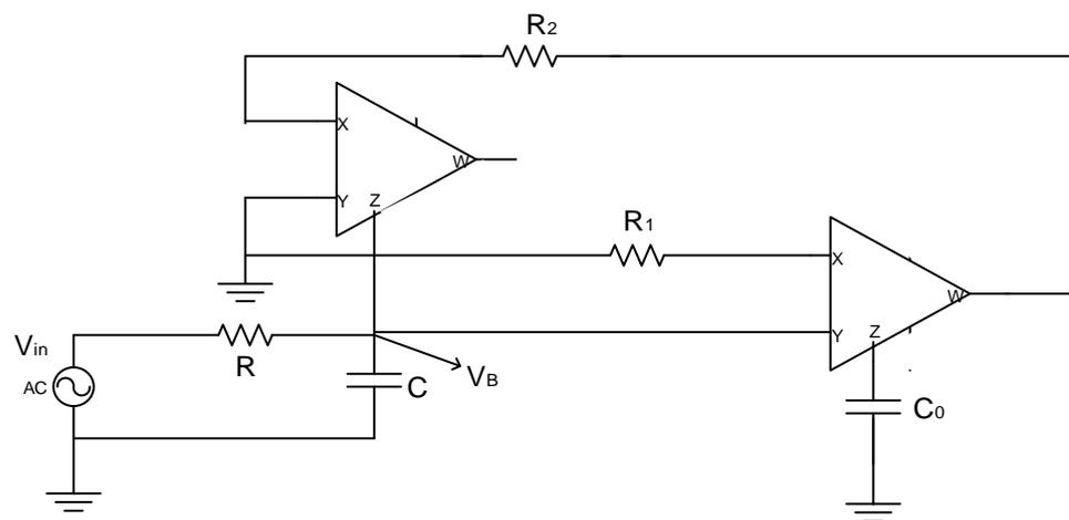
Fig. 4.18 Circuit diagram of band pass filter implemented using GIC.
