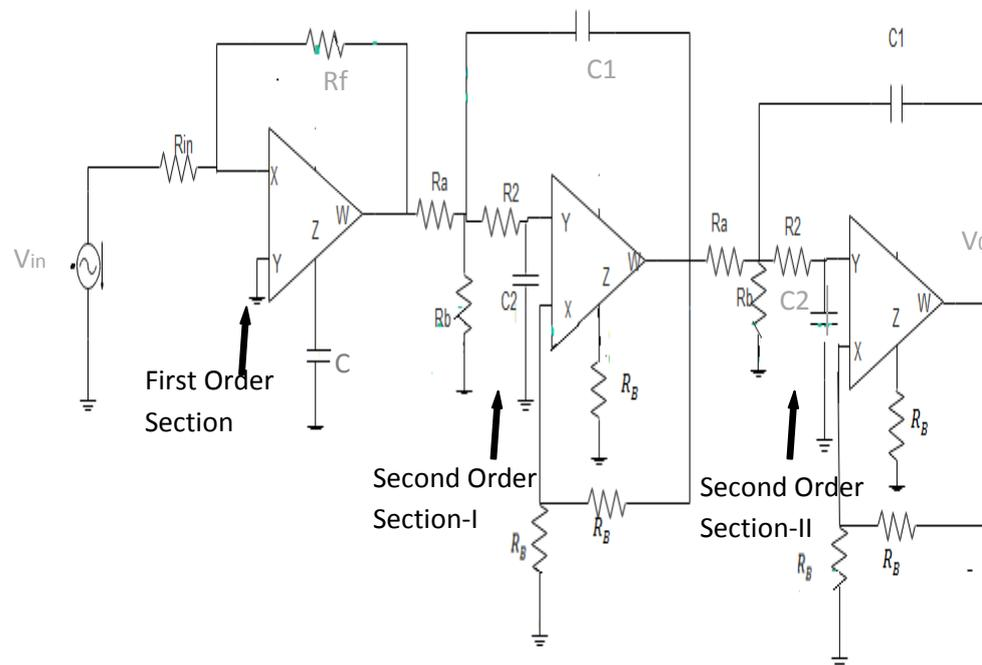
Fig 5.4 Fifth order Butterworth low pass filter circuit diagram
