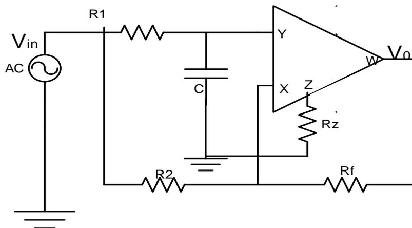
Fig 3.7 Circuit Diagram of First Order All Pass Filter
