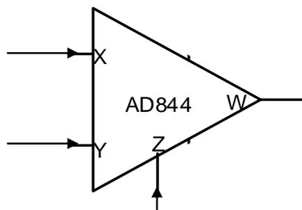
Fig 2.1 Functional Diagram of AD844 (CFOA)[14]
