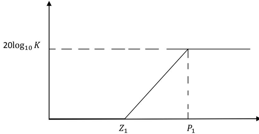
Fig 3.11 Ideal Characteristics of Bilinear Transfer Function with  $Z_1 > P_1$
