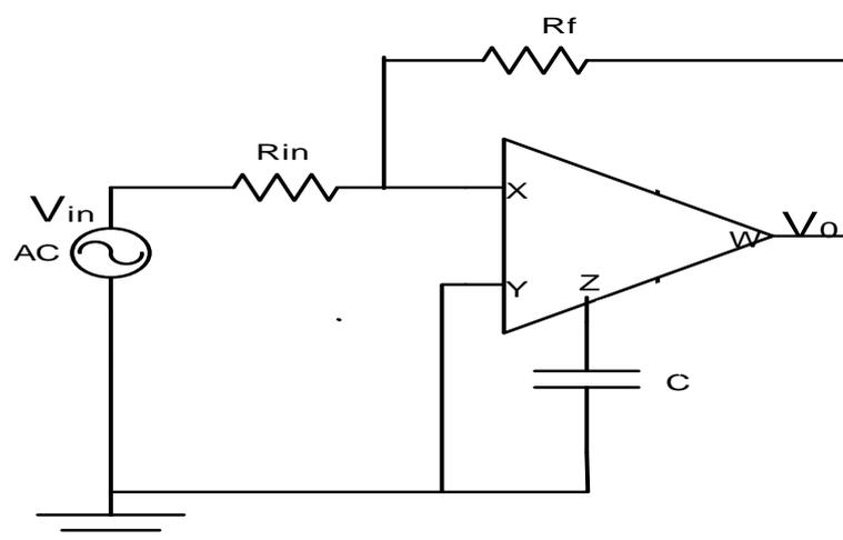
Fig 3.1 Circuit Diagram of First Order Low Pass Filter
