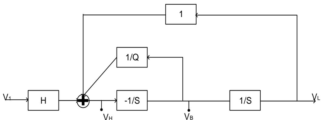
Fig. 4.10 Block diagram of Two Integrators in a Loop Biquad.[24]
