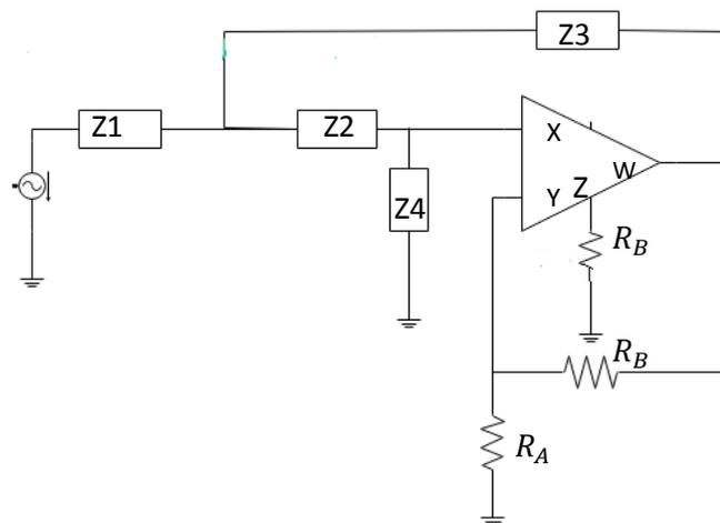
Fig 4.2 Circuit diagram of SALLEN-KEY configuration
