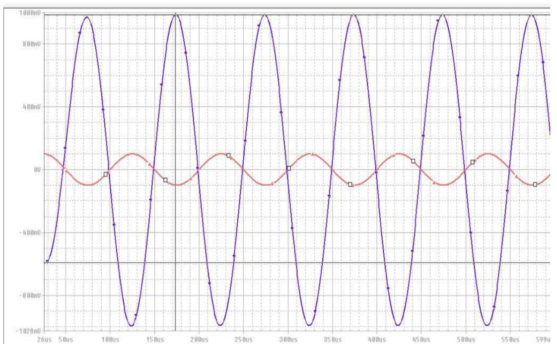
Fig 4.14 Transient response of Tow Thomas Biquad implementing band pass and low pass
