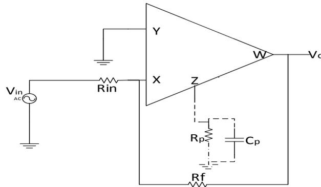
Fig 2.3 Circuit diagram of inverting amplifier
