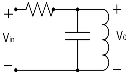
Fig. 4.16 Circuit diagram of Band pass filter
