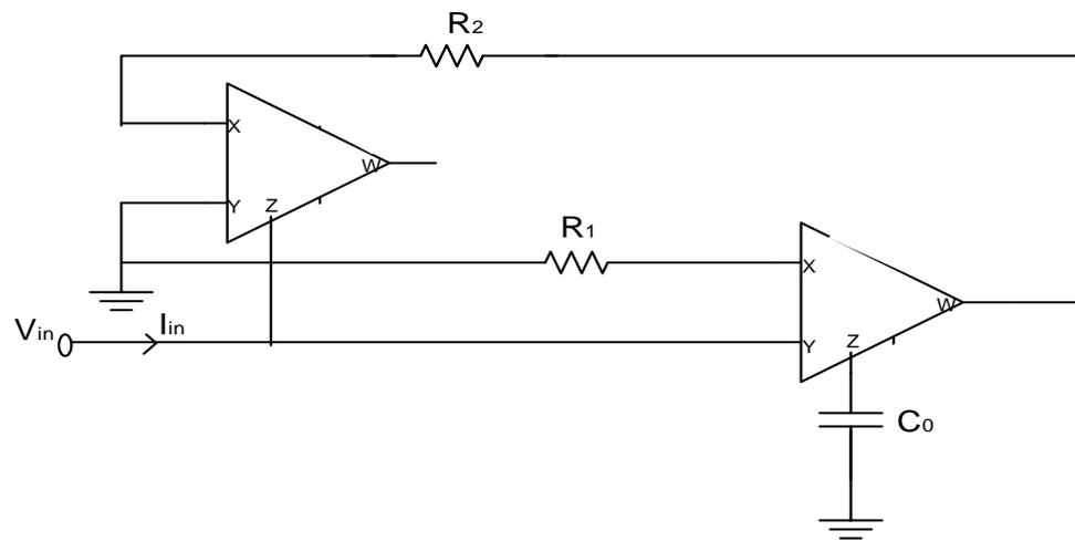
Fig. 4.15 Circuit diagram of grounded inductor
