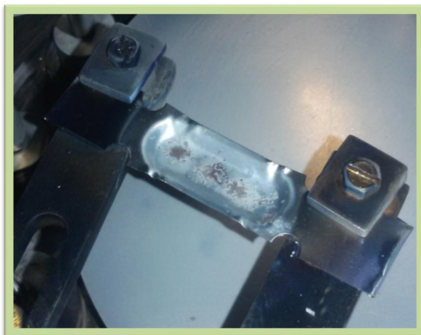
Figure 2.8 Boat containing \text{MoO}_3 fixed between two electrodes in a thermal evaporating system.
