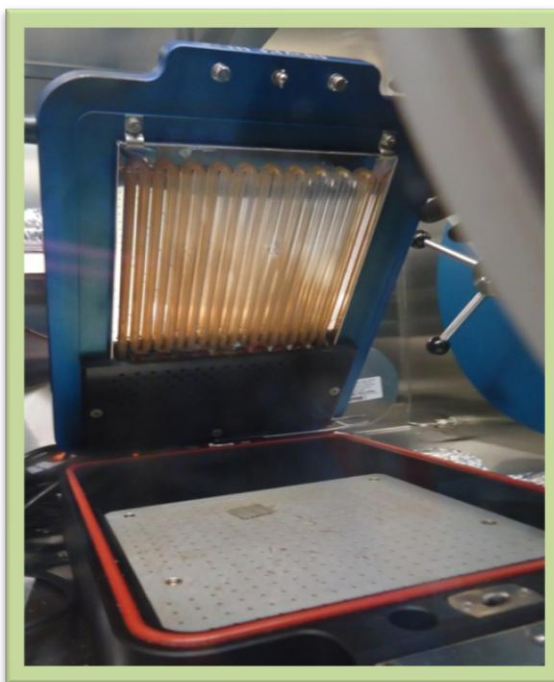
Figure 2.5 Photograph of UV ozone cleaner placed in glove box.
