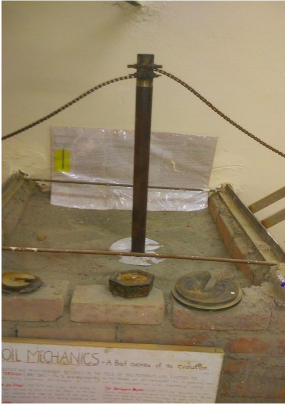
Fig 3.3: view of tapered pile inserted in The pit
