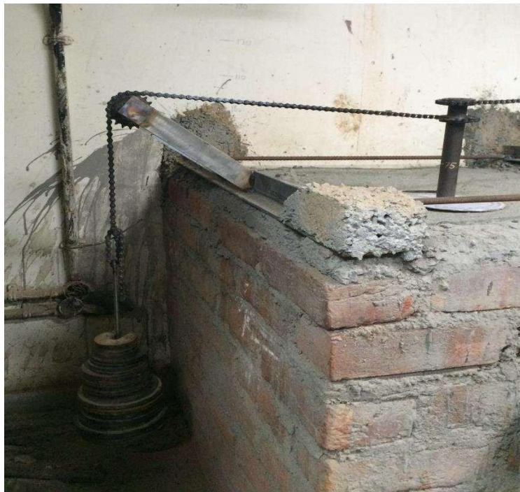
Fig3.9: chain in high tension carrying heavy load to apply torque on pile
