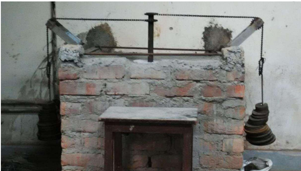
Fig3.14: elevation view of mechanism producing torque in pile
