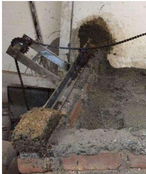
Fig3.2: girder fixed on top of brick wall and pulley inclined at 45° with vertical
