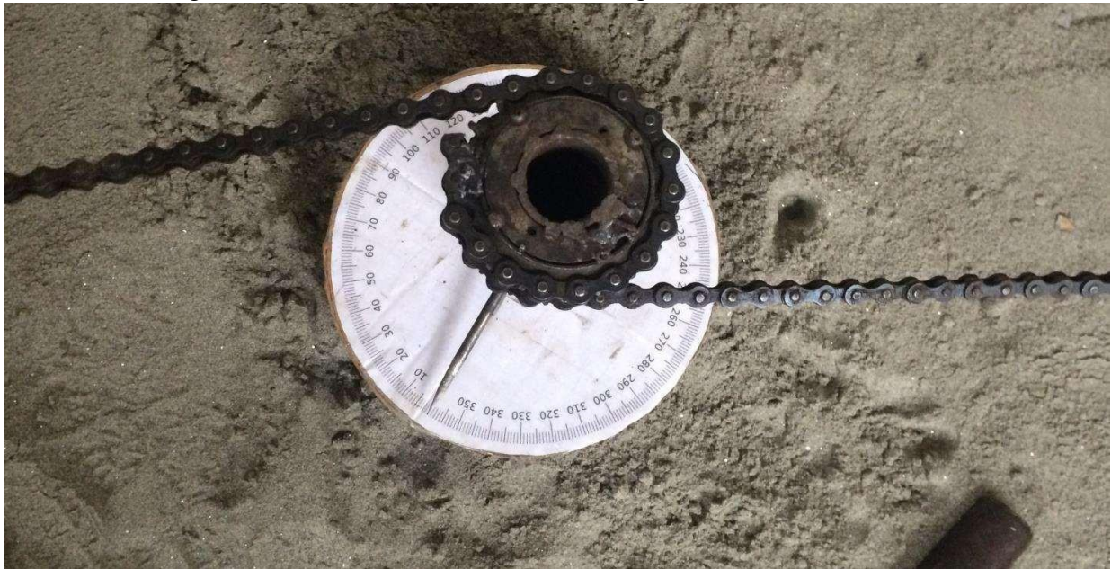
Fig3.12: calculation of angle of twist
