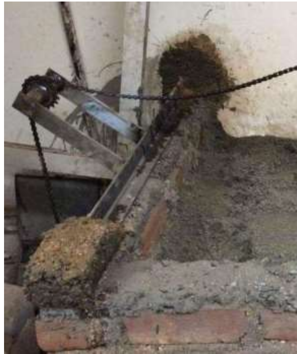
Fig3.4: girder fixed on top of brick wall and pulley inclined at 45^\circ with vertical
