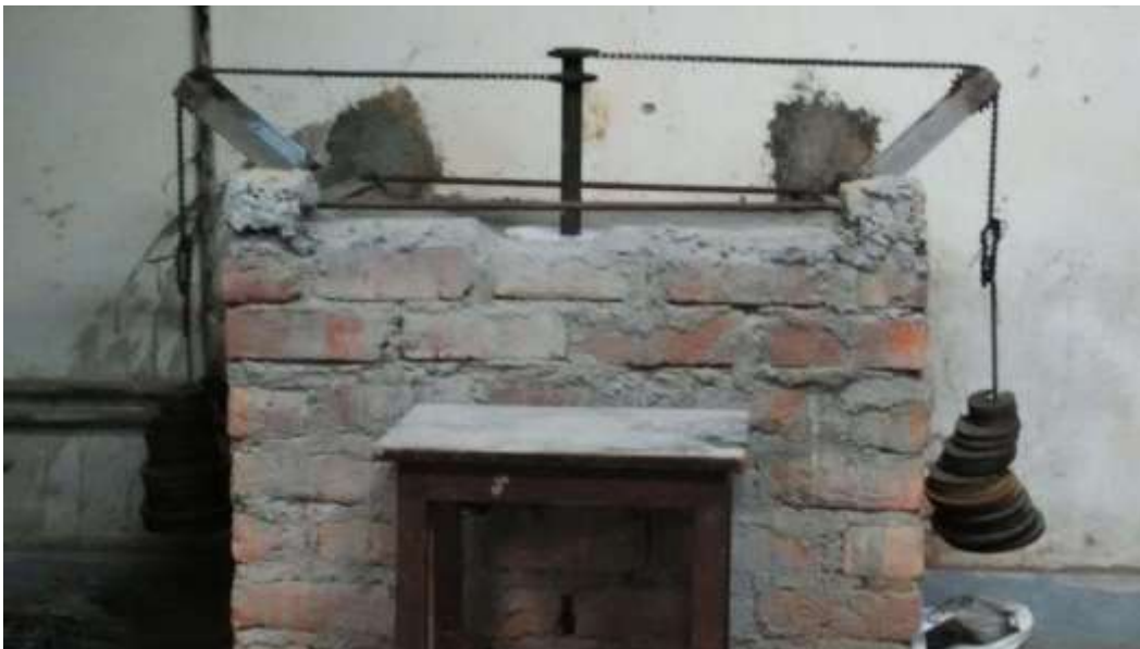
Fig3.13: elevation view of mechanism producing torque in pile
