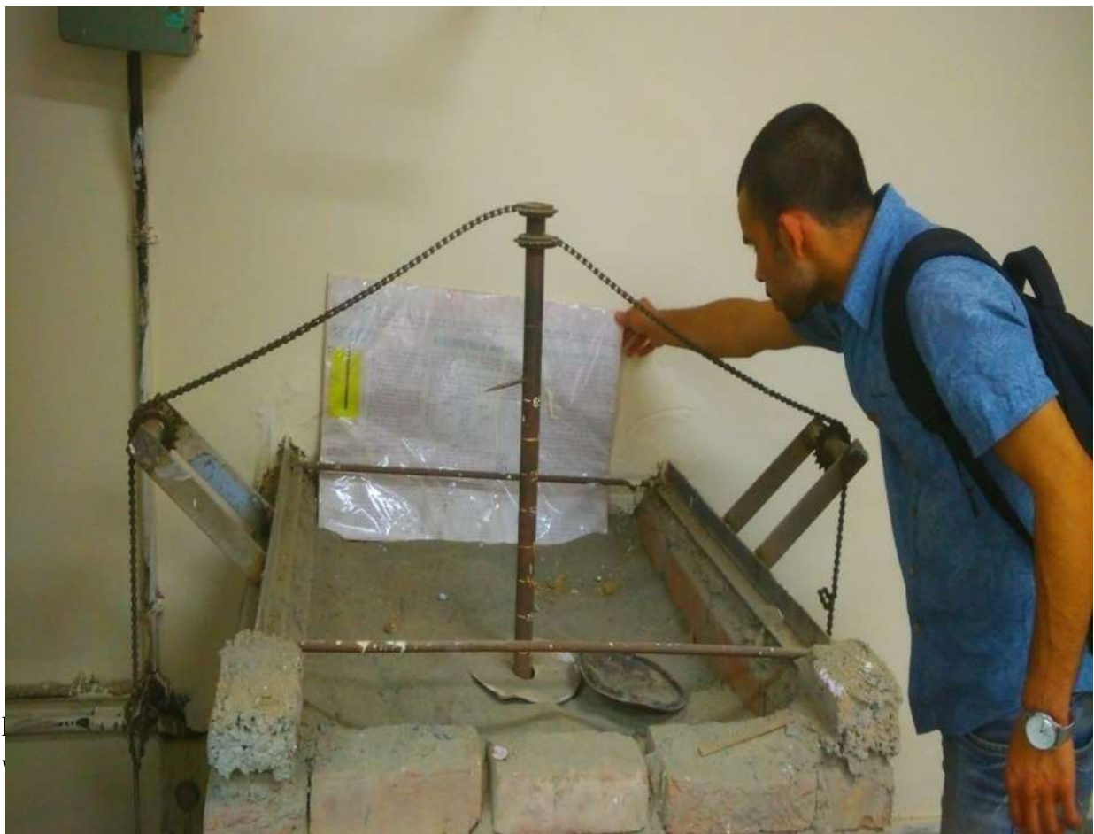
Fig3.4: girder fixed on top of brick wall and pulley inclined at 45^\circ with vertical
