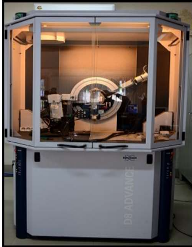
Figure 5.3: Bruker D-8 Advance XRD instrument.
