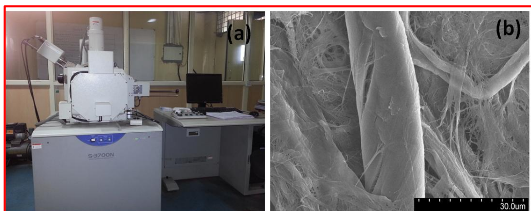
Fig. 2.11: (a) Optical image of SEM Hitachi model S-3700N and (b) SEM image of Whatman filter paper 1.
