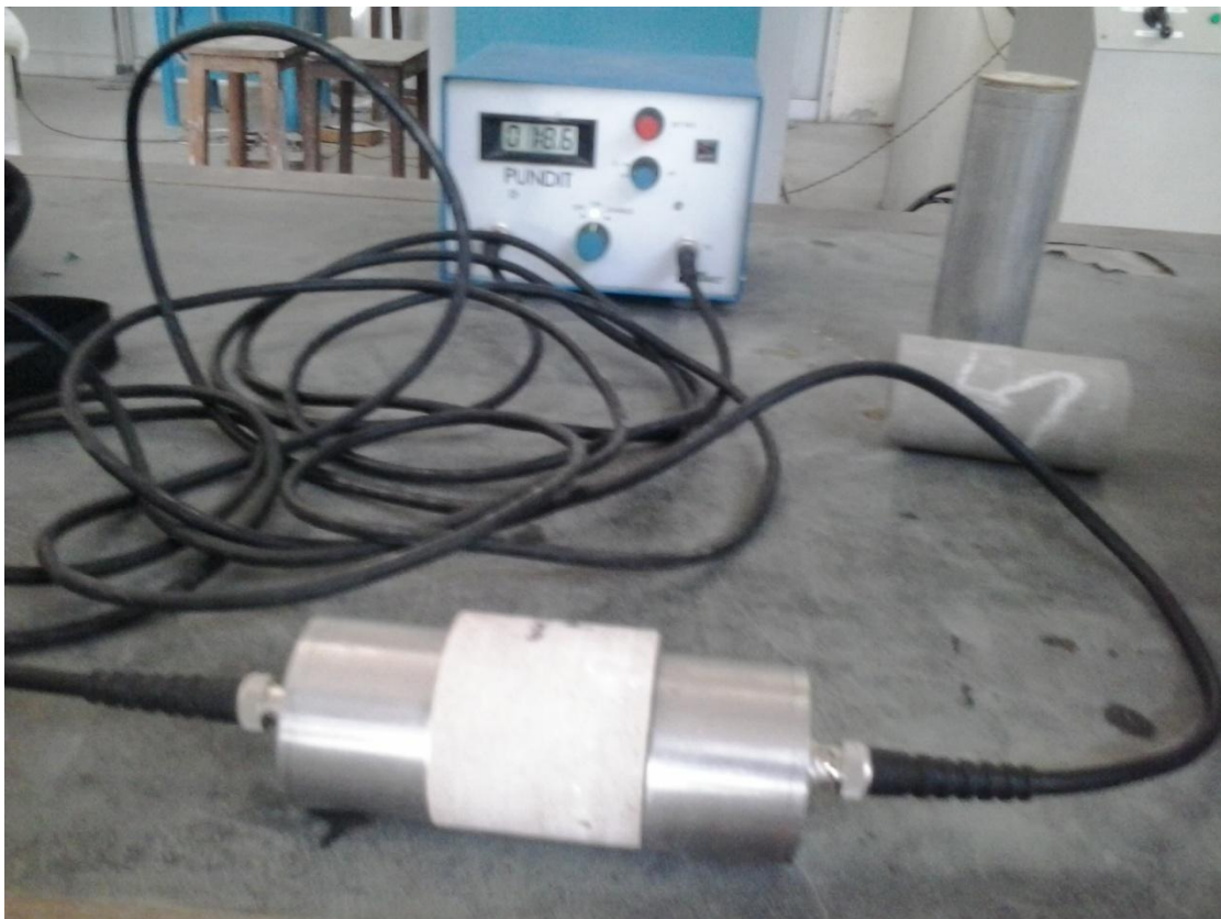
Fig 3.7 P-wave velocity determination in 50mm sample
