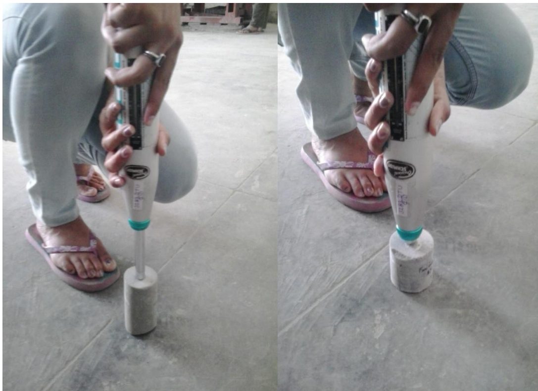
Fig.3.5. Determination of R value and compressive strength
