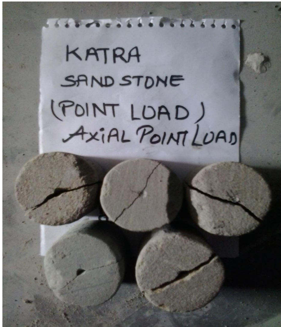
Fig 3.14 Failure pattern in sand stone
