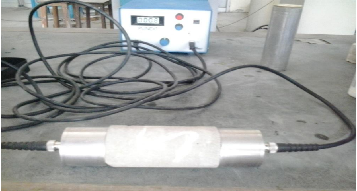
Fig 3.6 P-wave velocity determination in 100mm sample
