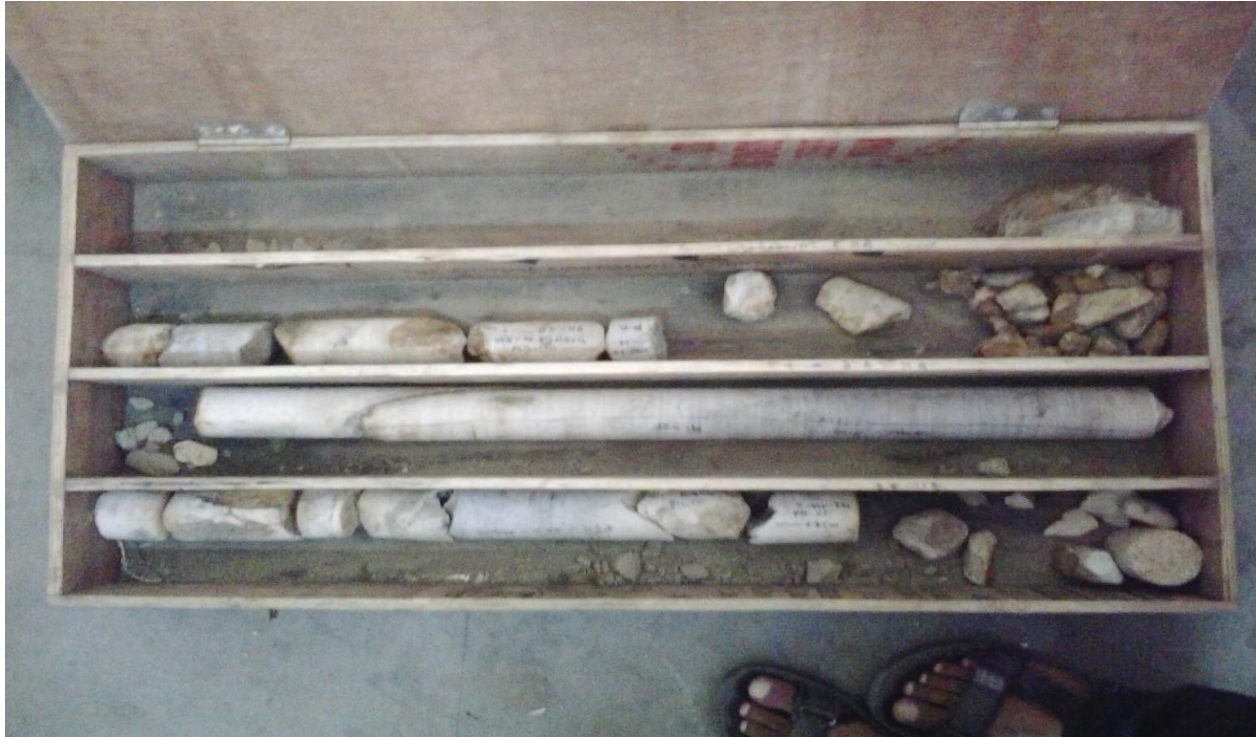
Fig. 3.3 Rock Sample for RQD (Faridabad)
