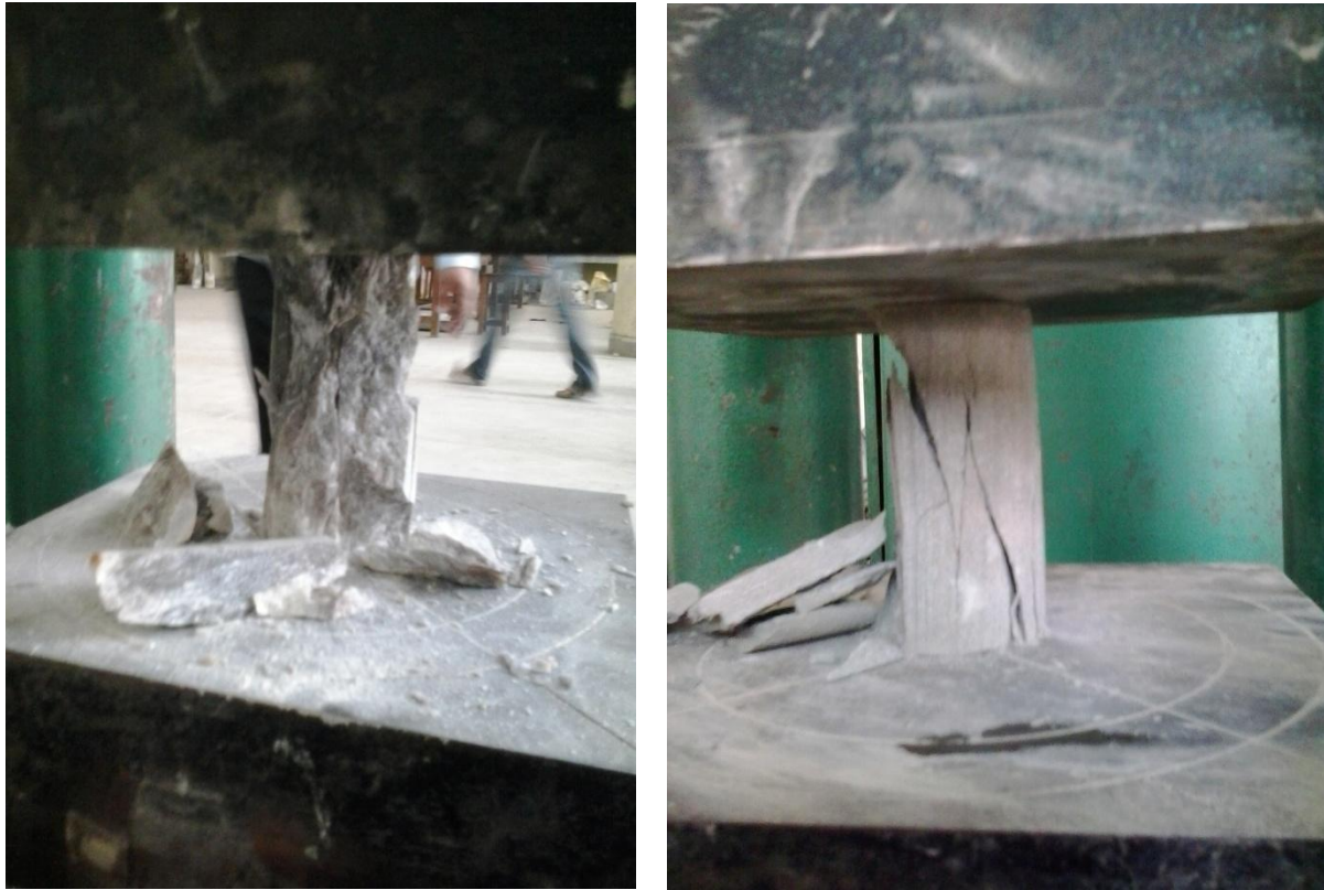
Fig.3.18 Failure pattern in unconfined compressive test
