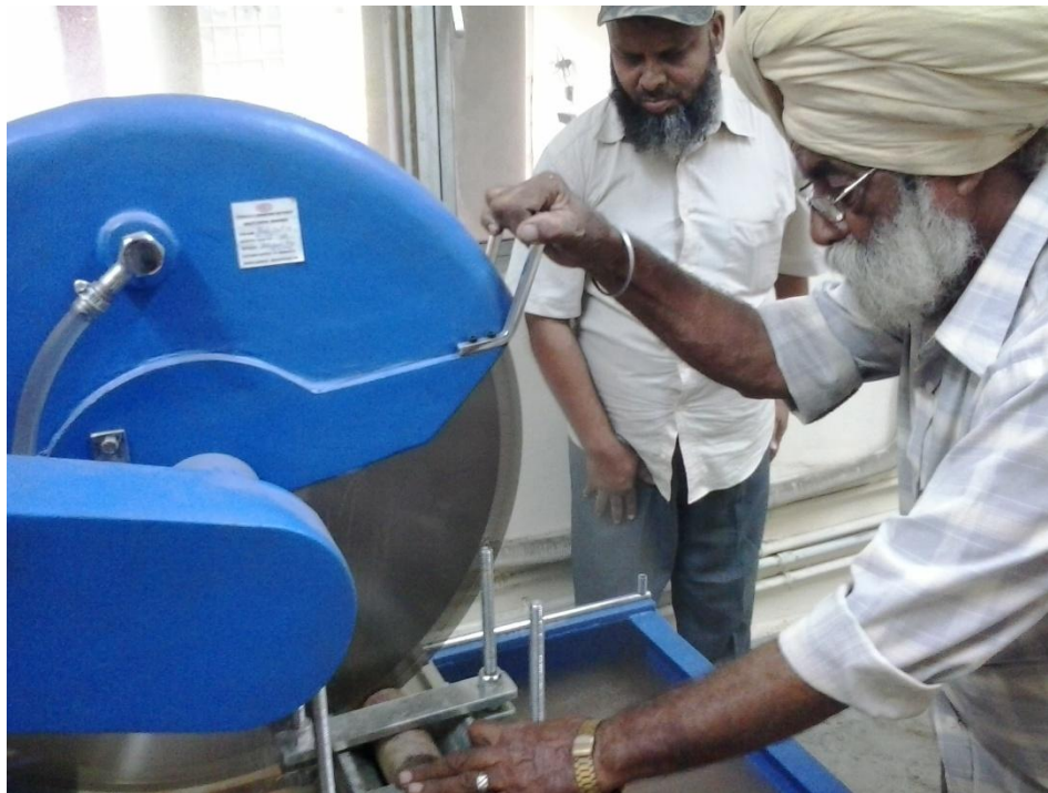
Figure 3.2 Preparation of rock sample by rock cutting machine
