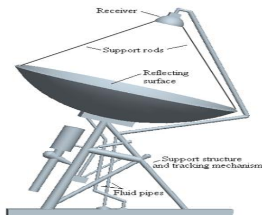
Figure21:- paraboloid concentrating collector (source:- Solar energy book)
