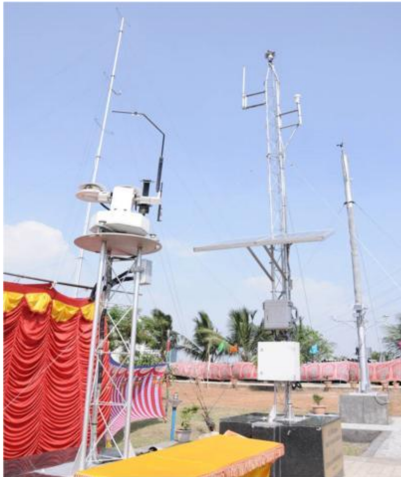
Figure14:- Solar radiation resource assessment (SRRA) station (source:- NIWE)
