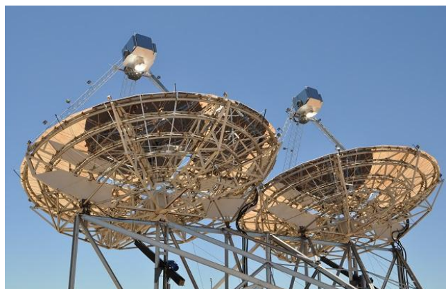
Figure30:- Cavity Receiver of solar Paraboloid Dish (source: - NREL)
