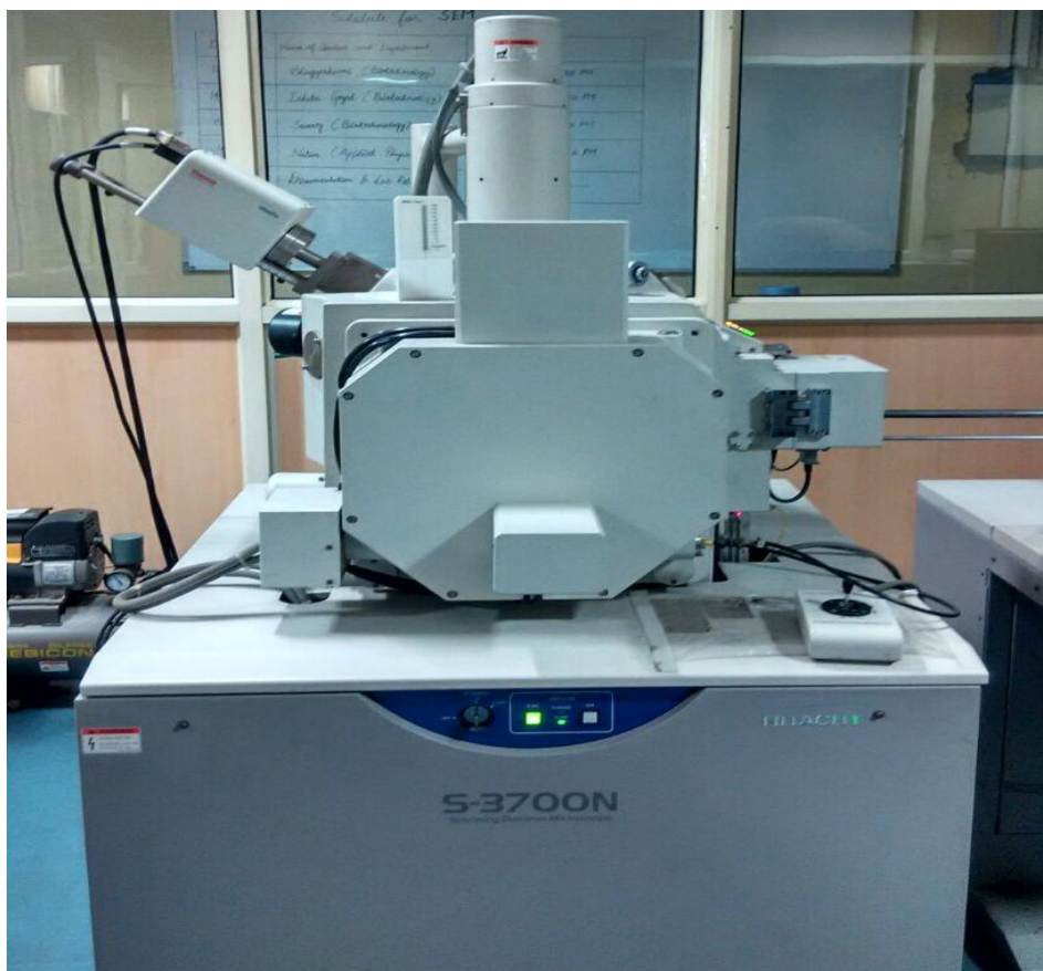
Fig.14. Scanning Electron Microscope (SEM) with attached EDX systems at Advanced Instrumentation Center, DTU.
