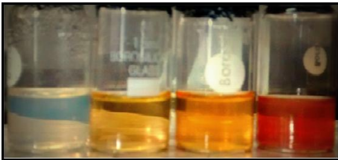
Fig. 8. Change in the colour of the solution with time when Plant extracts are added to silver salt.
