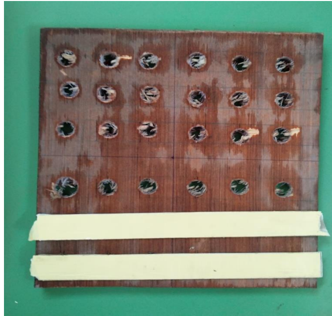
Fig 4.6 Perforated type (II) baffle wall with bottom two rows blocked
