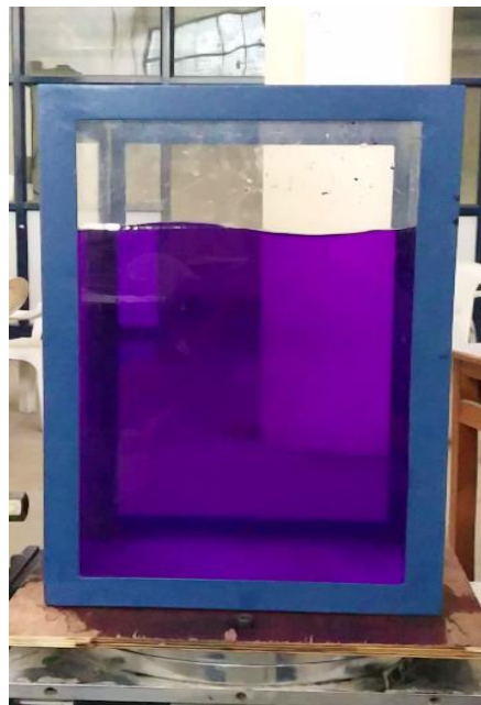
Fig 4.13 Shape of standing wave at Mode 2(75%) at frequency of 2.8 Hz
