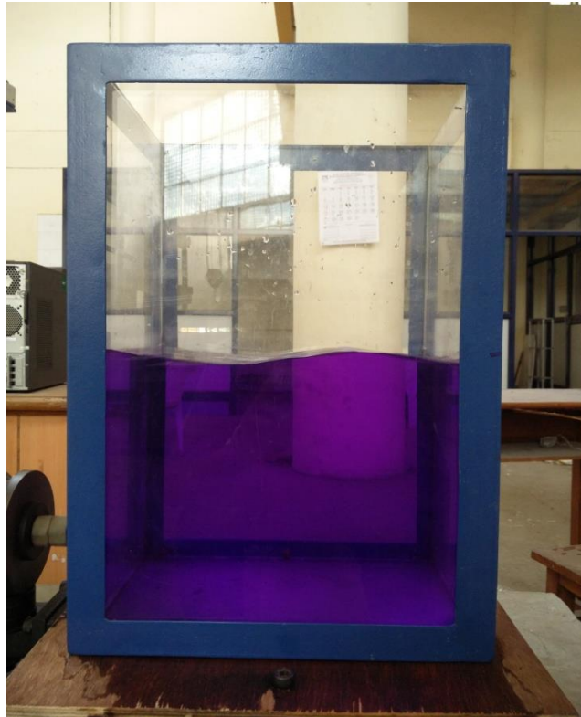
Fig 4.9 Shape of standing wave at Mode 2 at frequency of 2.8 Hz
