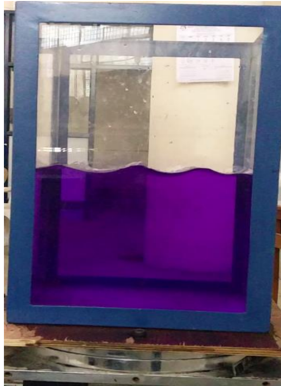
Fig 4.11 Shape of standing wave at Mode 4 at frequency of 4.4 Hz
