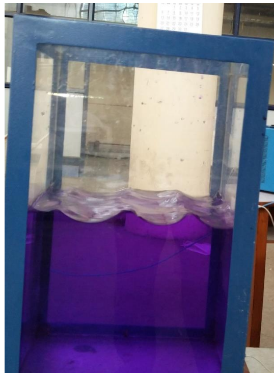
Fig 4.10 Shape of standing wave at Mode 3 at frequency of 3.7 Hz
