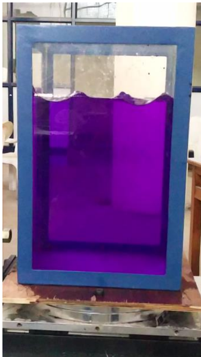
Fig 4.15 Shape of standing wave at Mode 3(75%) at frequency of 4.4 Hz
