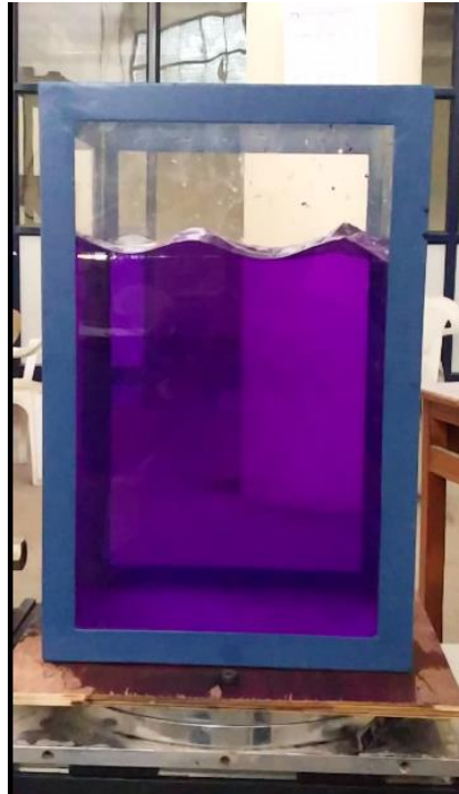
Fig 4.14 Shape of standing wave at Mode 3(75%) at frequency of 3.7 Hz
