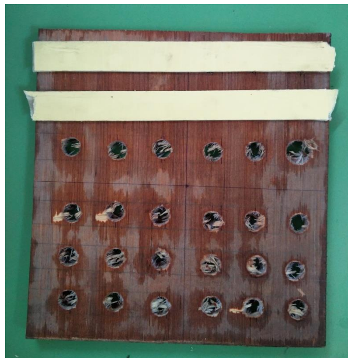
Fig 4.5 Perforated type (I) baffle wall with top two rows of holes blocked
