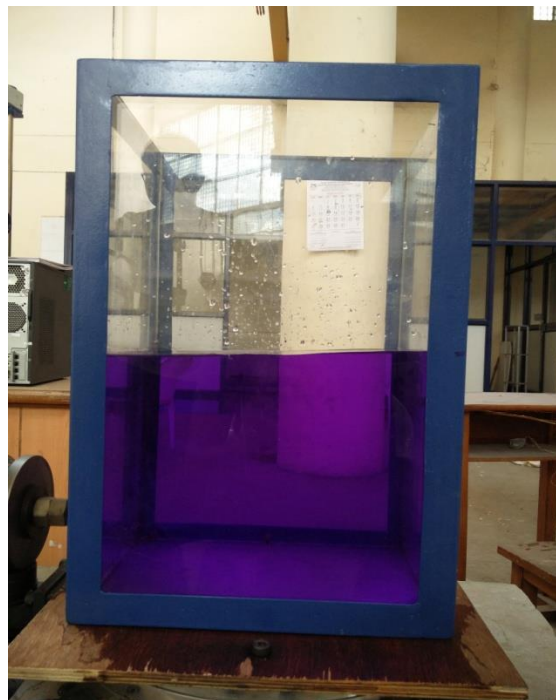
Fig 4.8 Shape of standing wave at Mode 1 at frequency of 1.6 Hz
