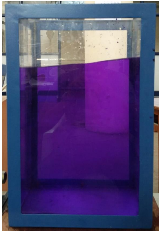
Fig 4.12 Shape of standing wave at Mode 1(75%) at frequency of 1.6 Hz
