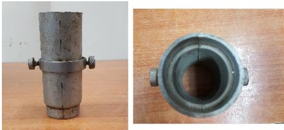
Figure 14 Sampler used for taking sample
