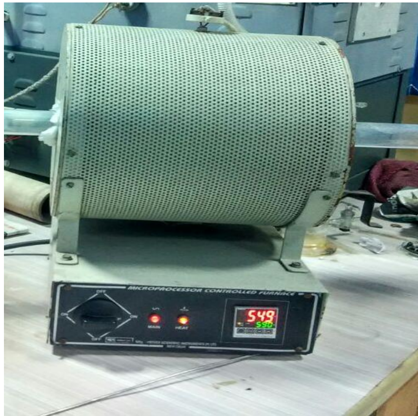
Figure 6.3. Picture of CVD Furnace used for experimentation
