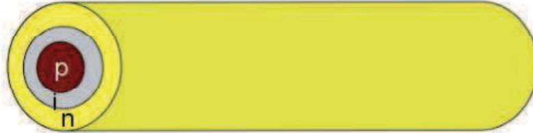
p-i-n configuration of silicon nanowire solar cell
