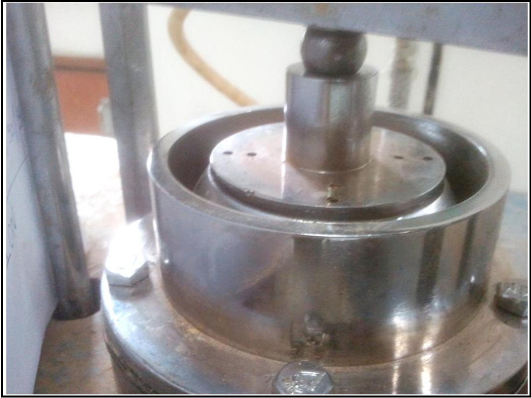
Fig 4.9: Parts of Consolidometer assembled
