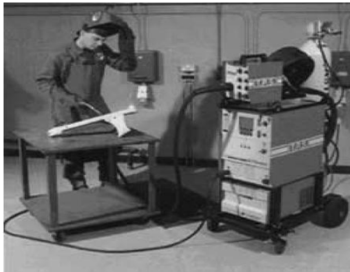
Fig3.2 Illustrating the general arrangement of the power source, wire feeder gas cylinder and work area, Courtesy of TWI Ltd.
