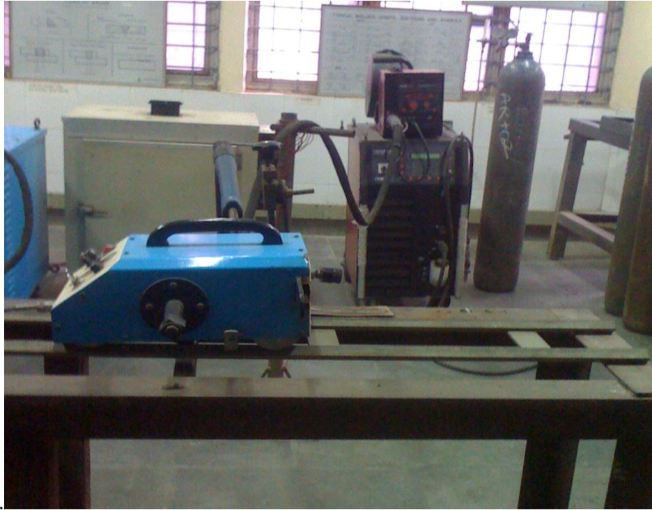
Fig3.9. Experimental set up for Synergic MIG Welding
